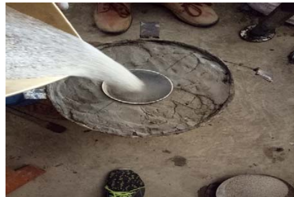
Figure 2 charging of pond ash
